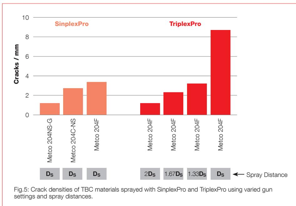
Fig.5: Crack densities of TBC materials sprayed with SinplexPro and TriplexPro using varied gun settings and spray distances.
