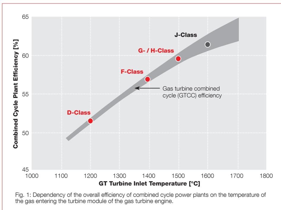
Fig. 1: Dependency of the overall efficiency of combined cycle power plants on the temperature of the gas entering the turbine module of the gas turbine engine.
