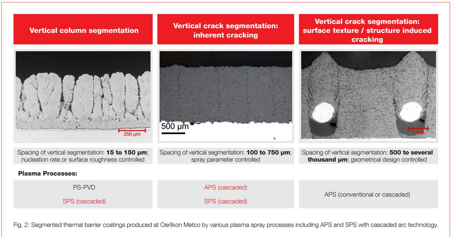
Fig. 2: Segmented thermal barrier coatings produced at Oerlikon Metco by various plasma spray processes including APS and SPS with cascaded arc technology.
