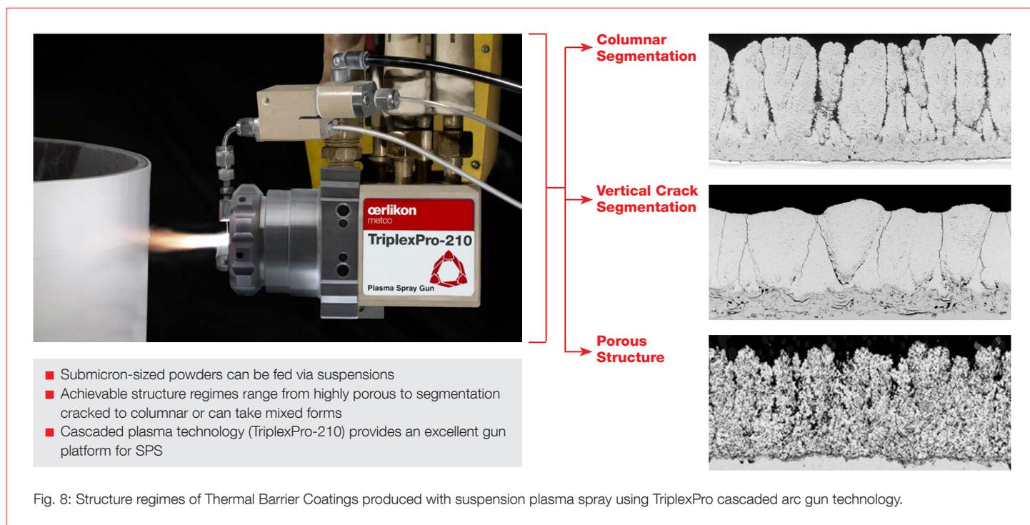
(usually ethanol). In the case of SPS, the segmentation can be in the form of cracks or columns as shown in Fig. 8, which shows the structure regimes possible with the SPS process and using the TriplexPro-210 gun.
