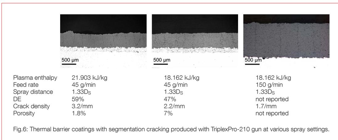
Fig.6: Thermal barrier coatings with segmentation cracking produced with TriplexPro-210 gun at various spray settings.
