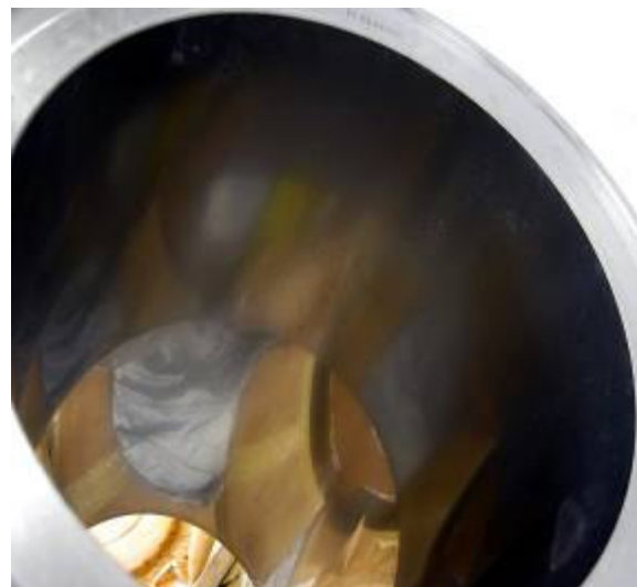
Figure 6: honed \text{\O}200\text{mm} SUMEBore coated cylinder liner with mirror finished surface
