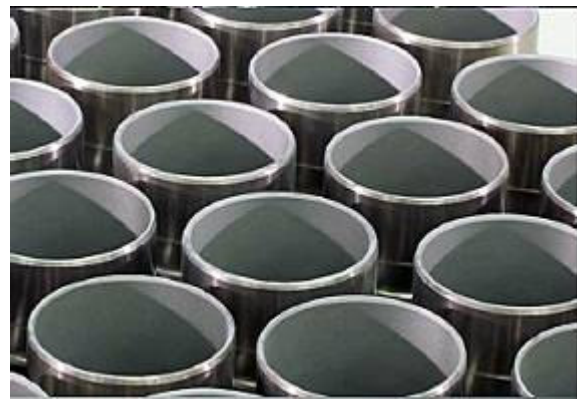
Cylinder liners from a truck engine, coated with rotating liner
