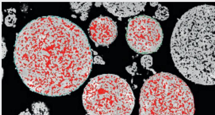
c) Low-k materials are better insulators than legacy 7–8 wt.% YSZ ceramics. Low-k materials have been developed for greater phase stability and service temperatures of more than 1200 °C (2192 °F). Metco 206A is an agglomerated and sintered low-k powder.
