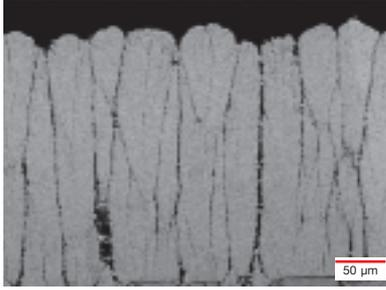
3 Sulzer developed PS-PVD processes to create improved TBC microstructures. The picture shows the cross section of a TBC sprayed with Metco 6700.
