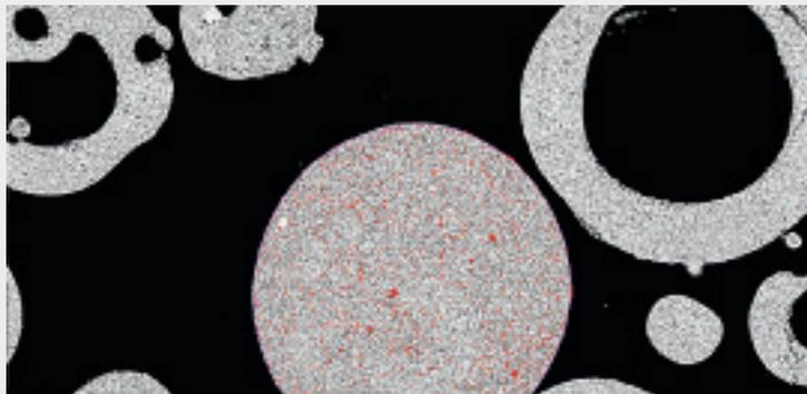
b) High-purity zirconia-based powders have been developed in response to new customer specification requirements and show improved high-temperature sintering resistance due to low concentrations of alumina and silica. Metco 222A is an agglomerated and sintered, high-purity 7–8 wt.% YSZ powder.
