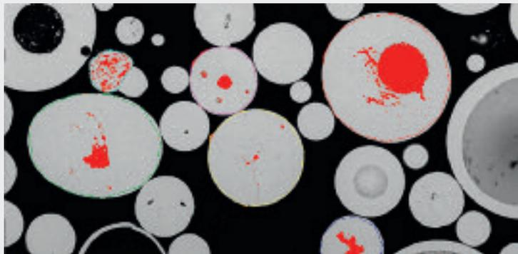
a) The Metco 204 product family includes plasma-densified hollow-oven spherical powders (HOSP™)/7–8 wt.% YSZ.
