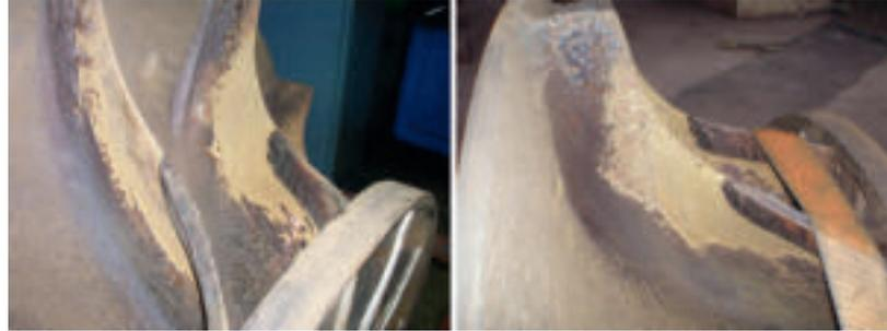
1 The impeller was eroded at its most turbulent locations in the flow path: blade tip, leading edge, and shroud.
