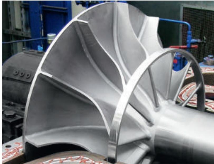
5 The measures of Sulzer slowed down the wear on the impeller vanes thus increasing the lifetime and—at the same time—decreasing the machine’s downtime.
