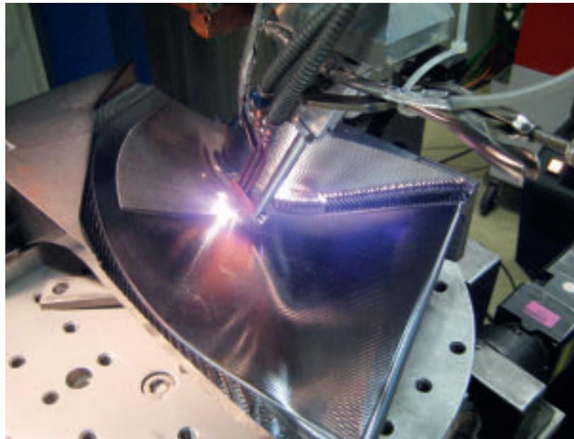
Of these solutions, only the Stellite welding gave encouraging results. However, the downside of the Stellite solution was that it was applied by hand arc welding, and therefore the resulting layer thickness and surface quality were inconsistent. Furthermore, it was difficult to apply the Stellite layer welding to larger surfaces.
