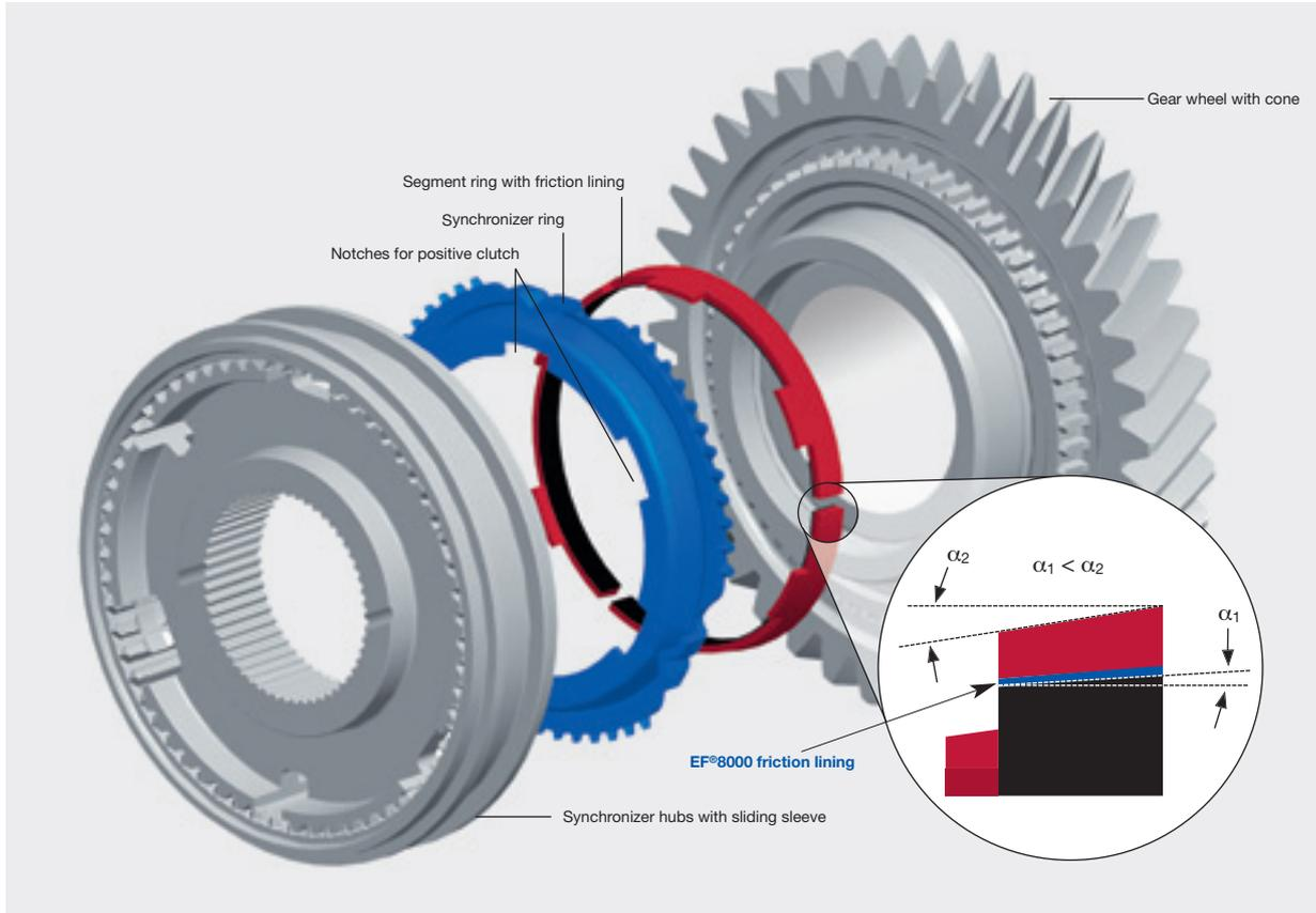
3 The new S<sup>3</sup> construction approach for segmented synchronization (blue and red components) sets itself apart in that the synchronous torque production and the release of the frictional contact are improved by being spatially separated and completely independent of each other (detail drawing).
