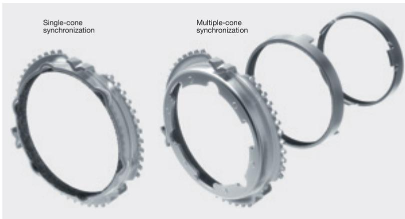
1 Synchronizers today are primarily constructed according to BorgWarner principles. Increased performance is achieved through multiple-cone synchronizations, which have a greater weight.
