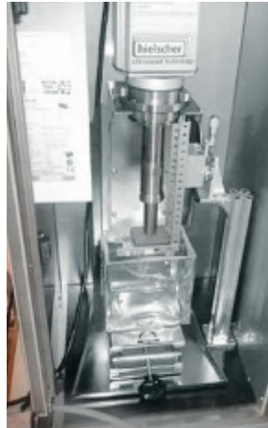
[8] Cavitation test rig at Sulzer Metco.
