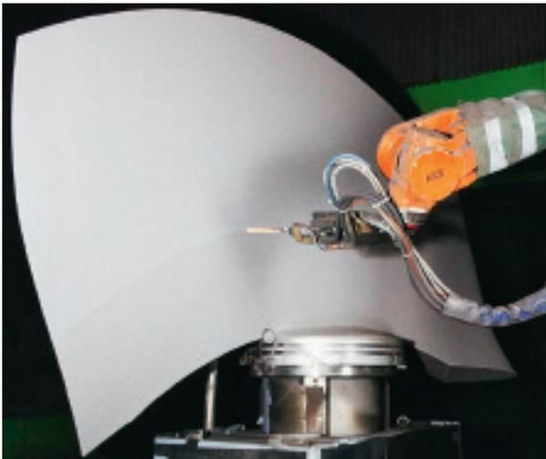
5 A Kaplan turbine blade, coated with Sulzer Metco SUME™Turb.
