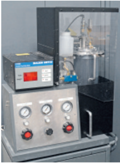
③ Liquid feed prototype system used to spray customer-driven applications.
