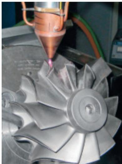
3 Rebuild of the tip of a turbocharger blade.
