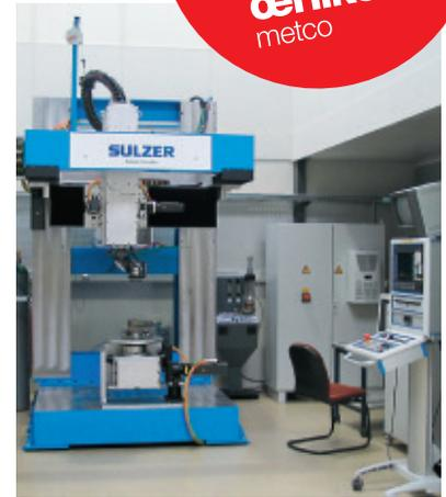
[2] Sulzer Innotec operates a gantry robot with a CO<sub>2</sub> laser and a fiber-laser system, which both support 5-axis simultaneous machining.
