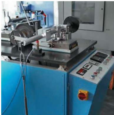
7 Oscillating test bench for the determination of adhesive and sliding abrasion under reversing conditions.
