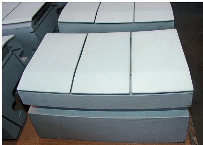
Oerlikon Metco's ceramic abrasible solutions, applied to 1<sup>st</sup> stage HPT shroud segments, are proven to increase overall efficiency by > 1 %.
