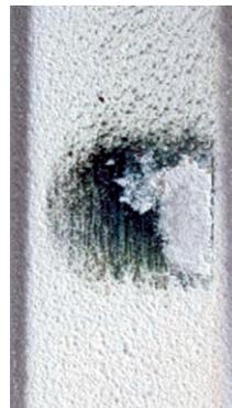
Mixed coating rupture and blade material transfer
