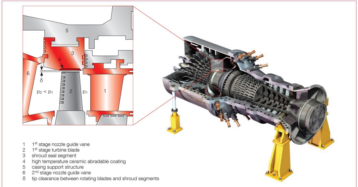
The abrasible ceramic seal materials are comprised of the ceramic matrix, a fugitive phase to control porosity and a release agent which enhances abrasibility. They are applied using atmospheric plasma spray such that porosity, erosion
