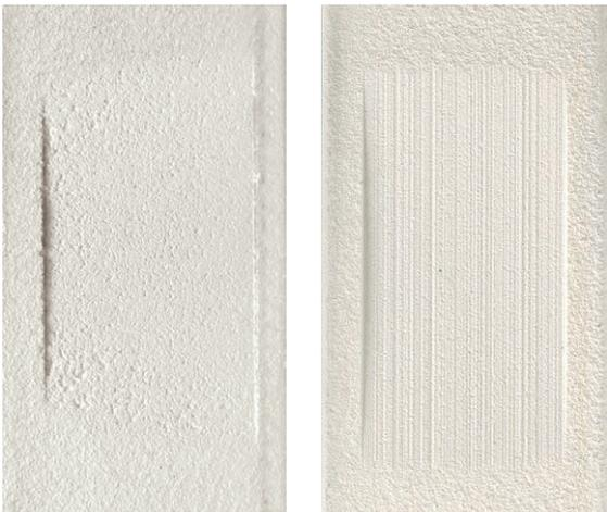
Examples of cleanly cut ceramic abrasable coatings @ 1100 °C (2012 °F). Left: against an un-tipped blade, Right: against a cBN tipped blade
