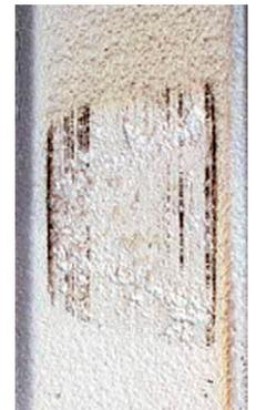
Slight coating rupture mixed with cutting and some blade material transfer
