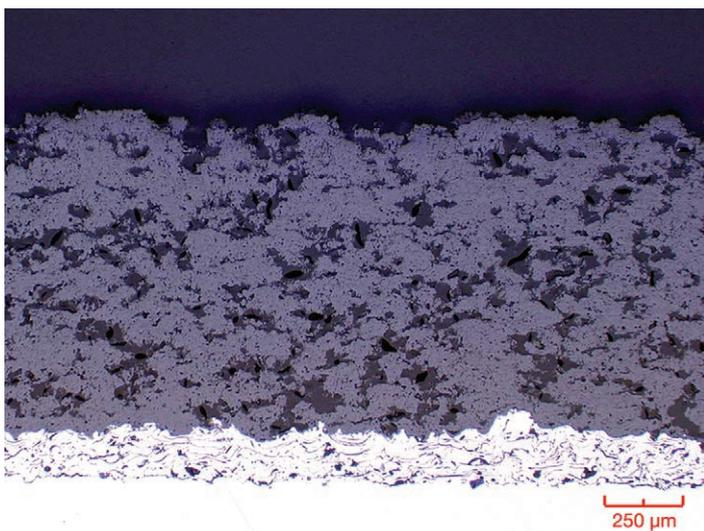
Typical microstructure of a high temperature ceramic abrasible, shown over an MCrAlY bond coat material.
