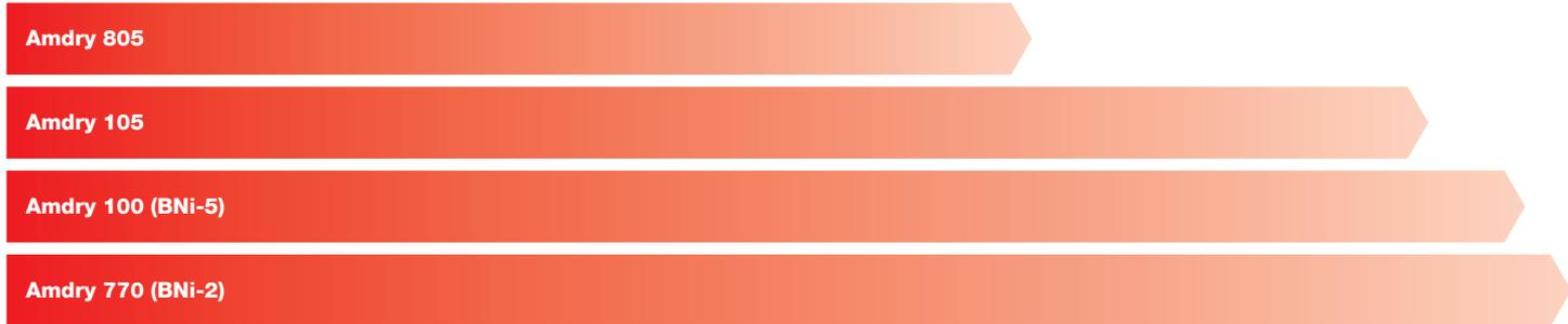
Comparative cost of Amdry 805 and Amdry 105 vs. traditional braze filler metals (Amdry 100 and Amdry 770).
