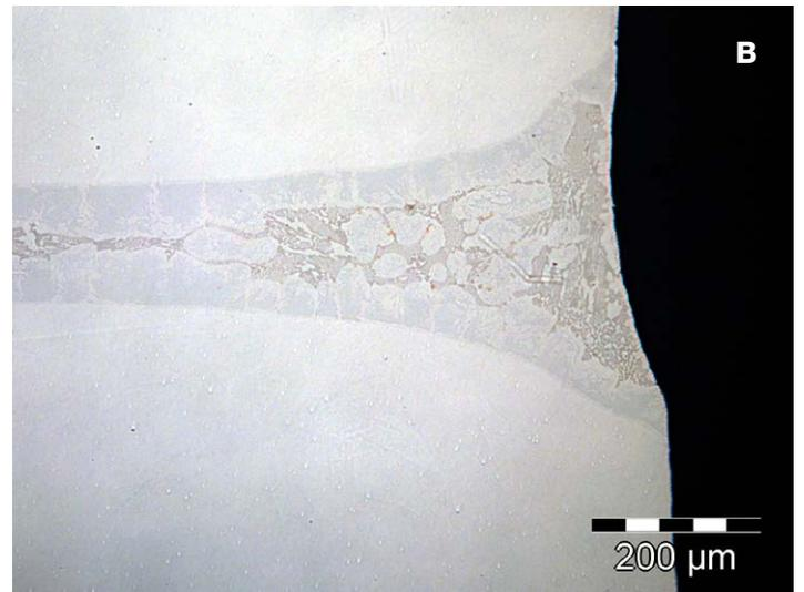
Photomicrographs showing examples of joints brazed with Oerlikon Metco's boron-free, reduced-nickel, high-temperature braze filler metals. A) Amdry 105, B) Amdry 805.
