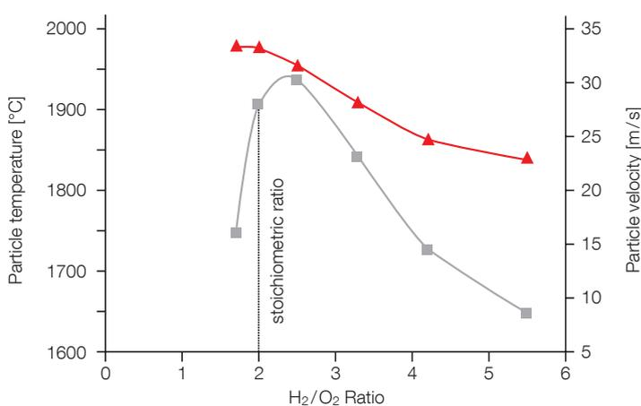
Real-time sensor technology was first used to establish the most stable area of the process window. In this case, it shows that a rich ratio of hydrogen to oxygen should be used.
