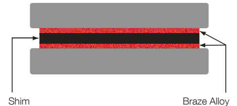
Figure 6. Wide-gap filled with base metal shim and braze alloy.
