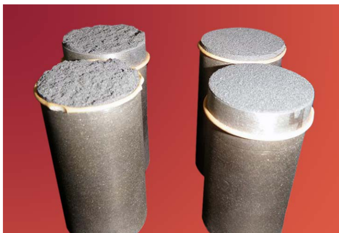
Figure 18: Left: linear coating fracture resulting from overheating during spray processing. Right: A properly temperature controlled coating results in a topographical fracture.
