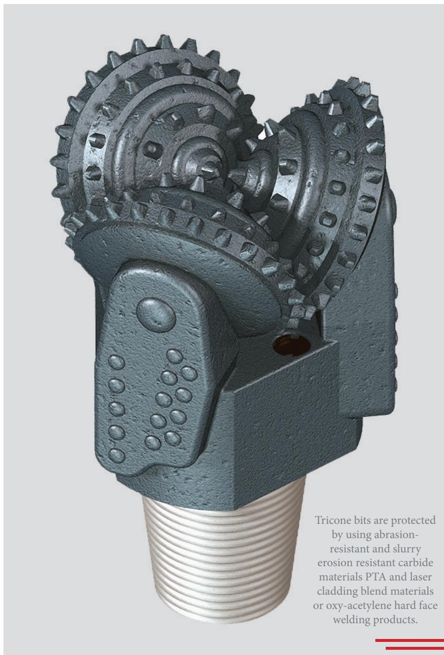
Tricone bits are protected by using abrasion-resistant and slurry erosion resistant carbide materials PTA and laser cladding blend materials or oxy-acetylene hard face welding products.
