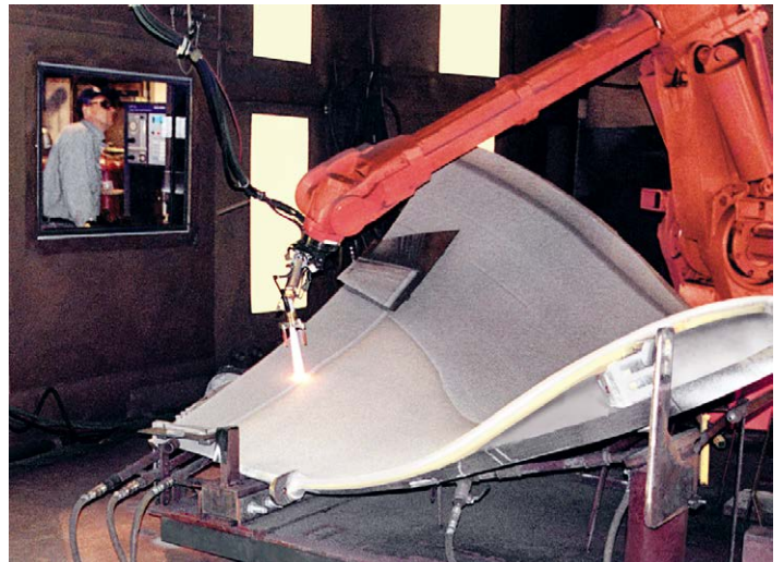
A large Kaplan runner blade being coated for service at a major dam project. The Metco TURB-coated blade will last up to 25 times longer than an uncoated blade.
