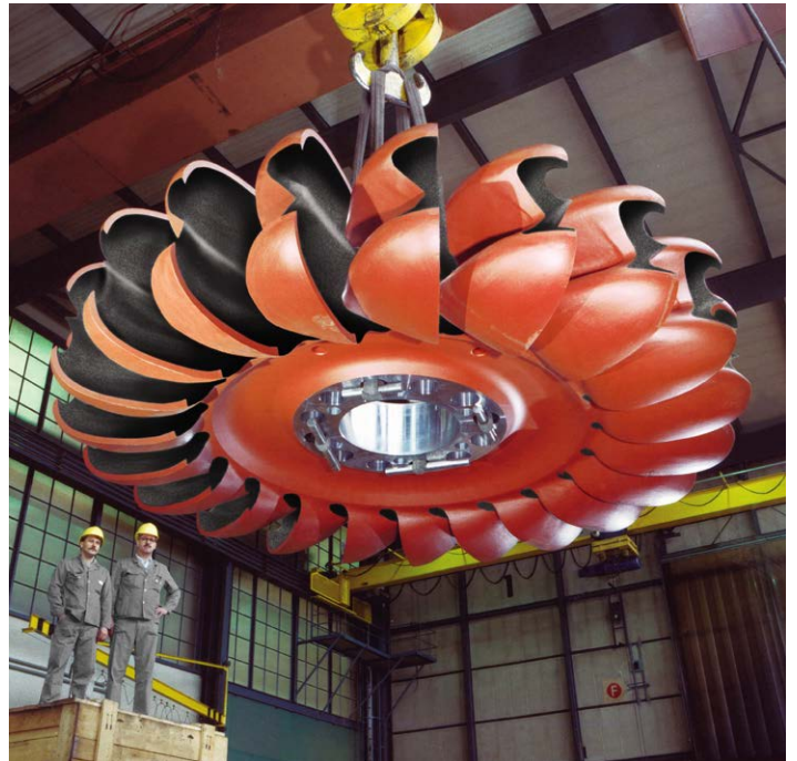
A large Pelton turbine wheel, just coated with Metco TURB will last up to 20 times longer than uncoated turbine wheels.
