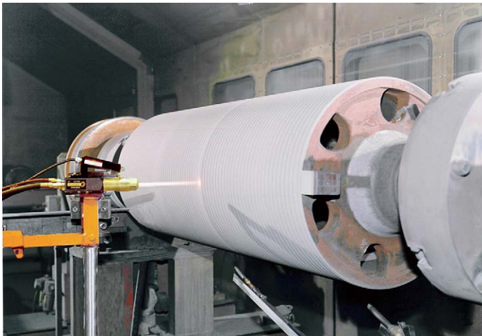
Coating a sink roll using a high-velocity oxy-fuel (HVOF) spray
