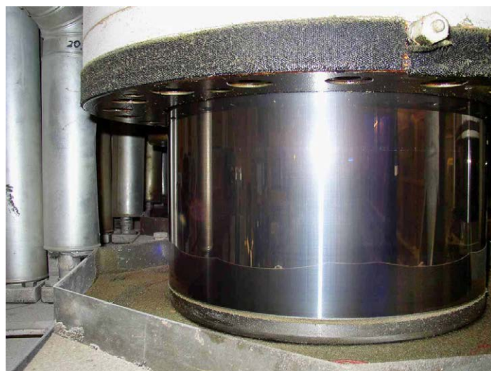
Coated hydraulic ram operating in a short-cycle press for the production of laminates
