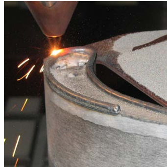
Turbine blade tip repair with MetcoClad 625
