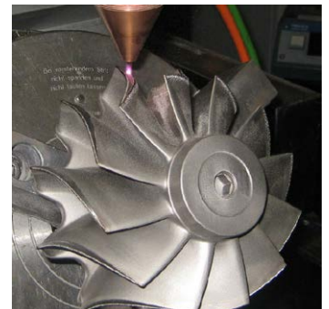
3D turbocharger blade tip repair with MetcoClad 625
