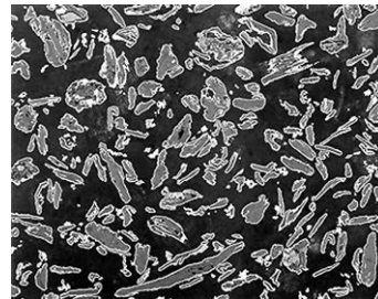
75% Ni / C 25% Original Magnification 200X D50 = 54 \mu m
