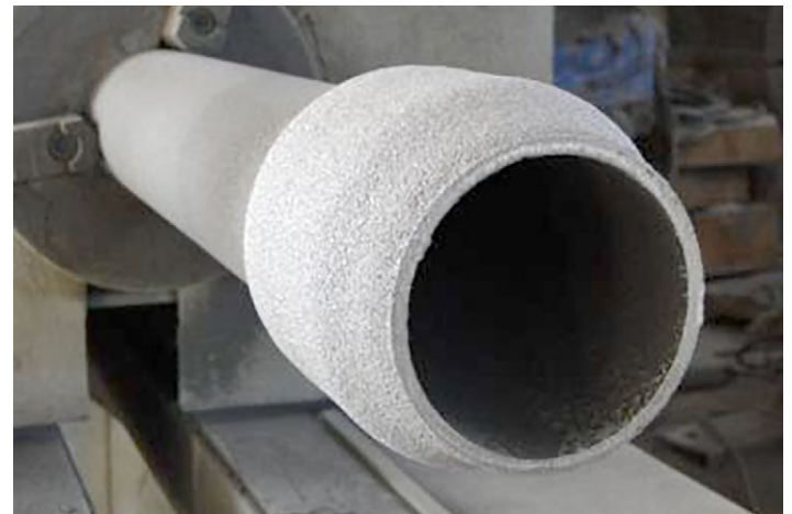
A thick coating of Metco 8280 hand-sprayed at a distance of 200 mm (8 in). Notice the light gray, metallic appearance of the coating. This is indicative of the low oxide microstructure of Metco 8280, which results in high bond strength and consistent coating quality.
