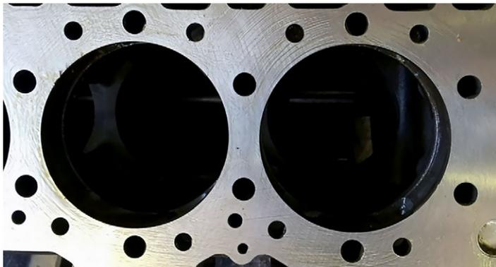
Engine deck restored with Metco 8293.
