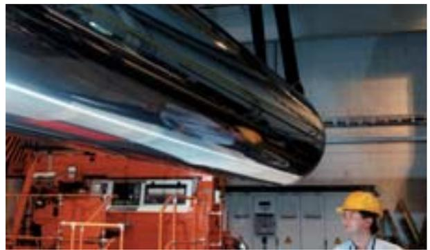
1 The surface of calender rolls has a significant impact on the quality of the paper. Coatings produced by Sulzer Metco ensure that a constant high level of quality can be maintained over a long period.
