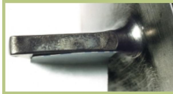
6<sup>■</sup> Although a coating in which the residual stress is compressive is normally superior in performance to one in which the residual stress is tensile, the coating system with the highest compressive stress (F-1) failed during a test under service conditions due to spalling of the coating.
