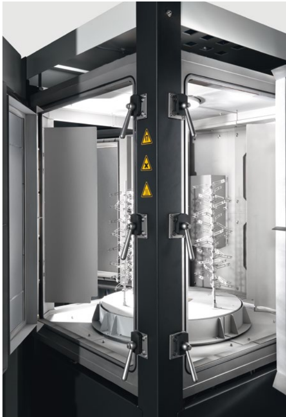
Triple door design of INUBIA B6 recipient
