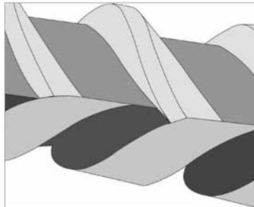
BALINIT® DLC for screw spindles shows significantly longer lifetime compared to nitride steel DIN 1.7131 in abrasive grinding cooling media.
