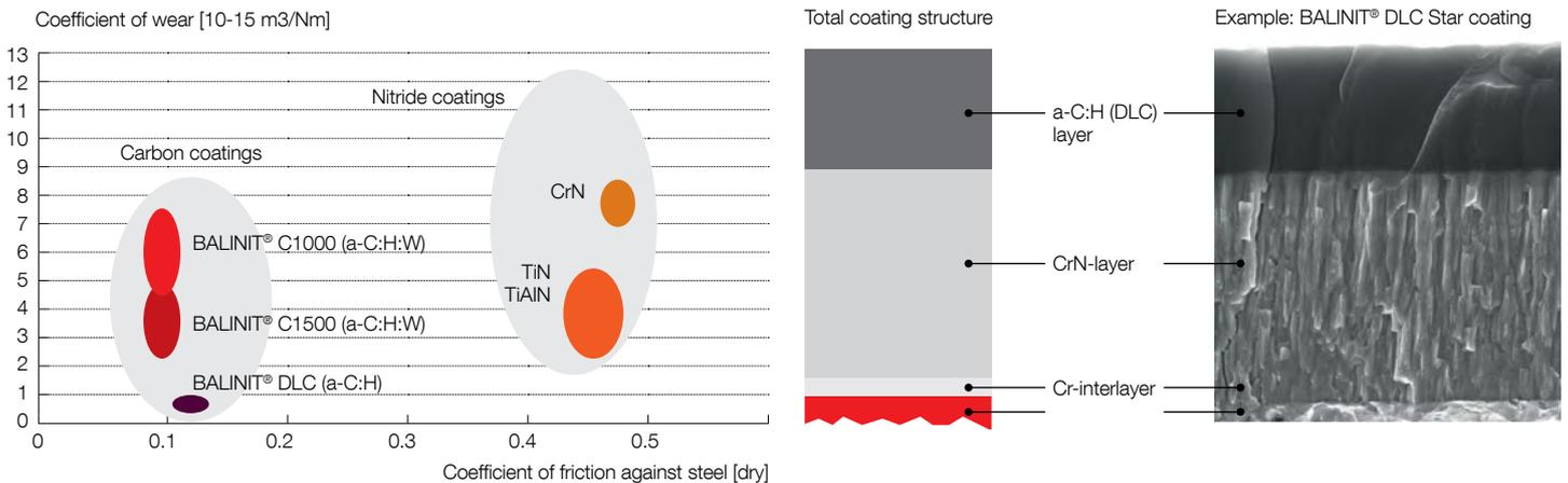
The abrasive wear resistance was measured by the ball crater method where a 20 mm ball rotates on the surface with continuous addition of diamond suspension. The friction is measured in a pin disk arrangement under dry condition against steel. Especially BALINIT® DLC and DLC STAR show a unique combination of low wear and low friction.
