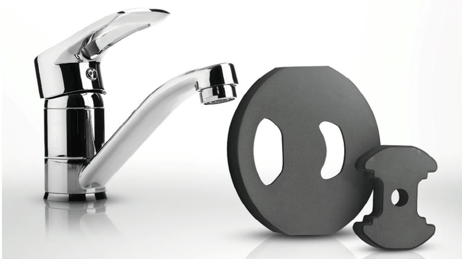
Extended service life: ceramic seal discs in sanitary fittings coated with BALINIT MILUBIA ensure a low operating force even when assembly grease is washed out after a long period of use.
