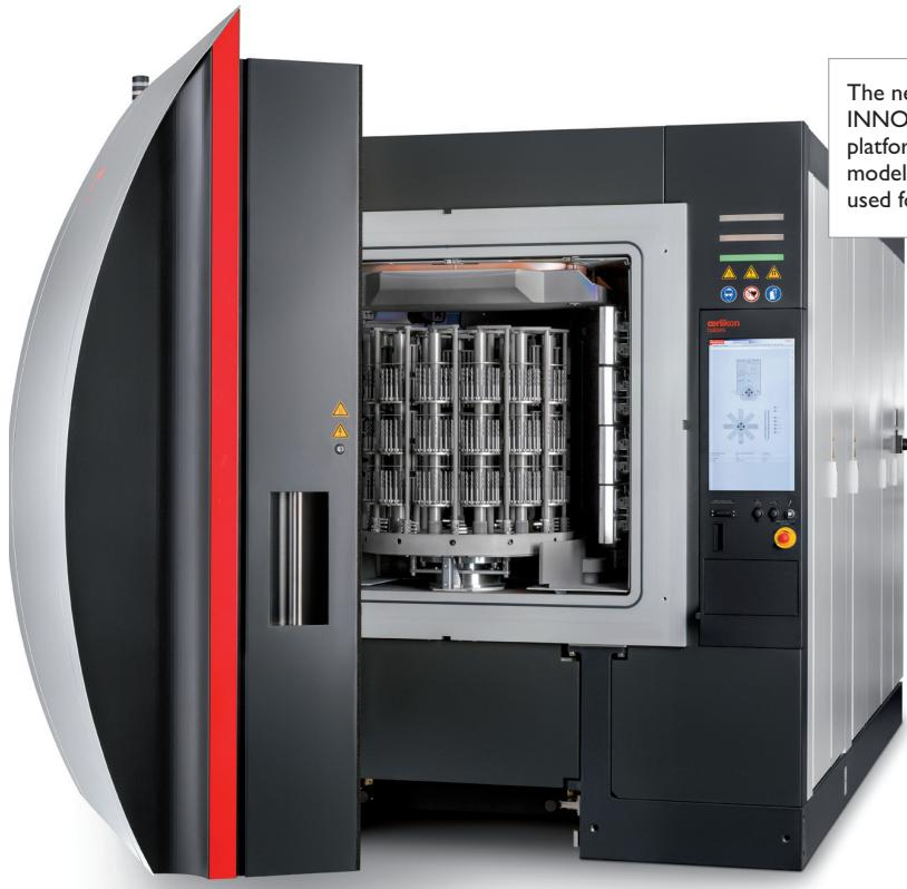
The new INNOVENTA kila is fully compatible with all other INNOVENTA family systems because it uses the same platform. The diameter of the carousels is the same for all models so that the holding and loading platforms can be used for the entire INNOVENTA family.
