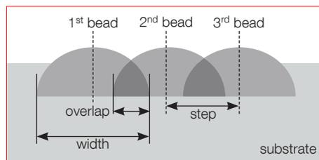
**Figure 1:** Graphical explanation of Step / Overlap / Width
