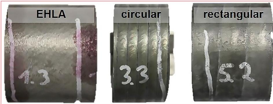
**Figure 5:** Surface topography of tubes after laser cladding
