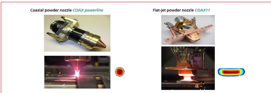
**Figure 5:** Examples of high power nozzles with circular and rectangular spots (Courtesty of Fraunhofer IWS)
