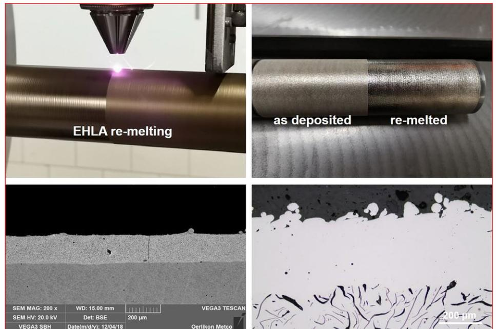
**Figure 3:** Surface quality after EHLA and re-melting; Cross-section of microstructure for Metco 15E (on the left side) and new generation Metco Fe-based alloy, deposited directly on cast-iron.
