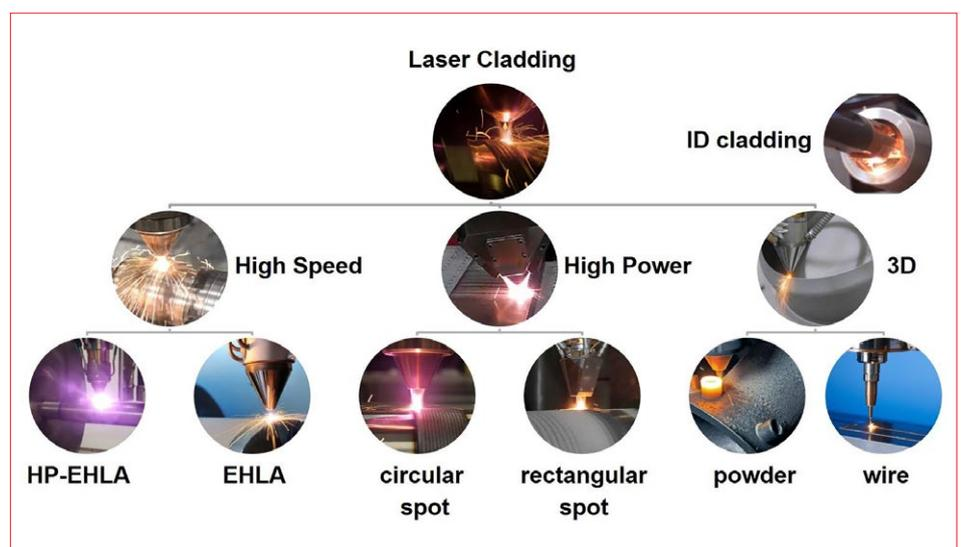
Figure 1: Classification of Laser Cladding
