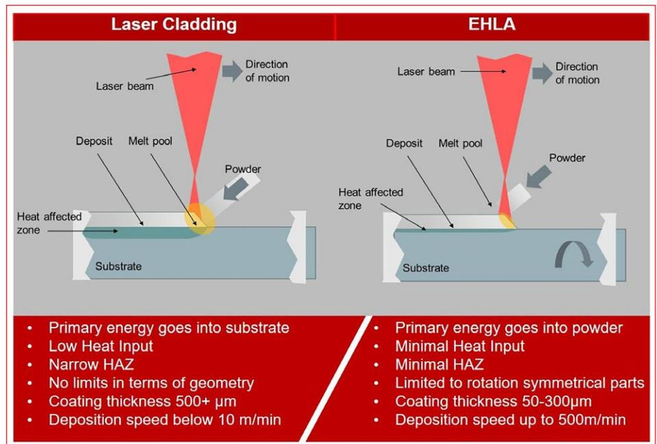
Figure 2: Laser Cladding vs EHLA
