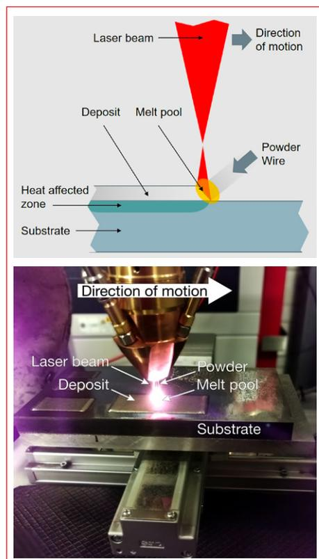
Figure 2: Laser Cladding Process
