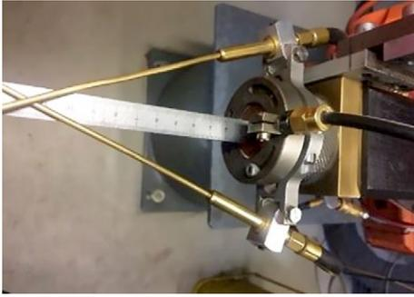
Figure 10: Setting up focused air-cooling jets.
