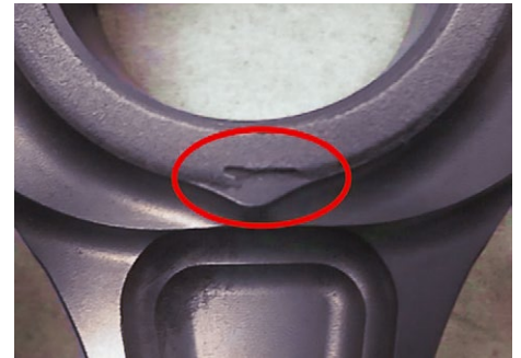
Figure 3: "Shadowed" APS molybdenum-based deposit.
