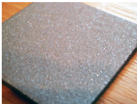
Figure 5: Typical appearance of a test panel grit blasted with 20 mesh alumina.
