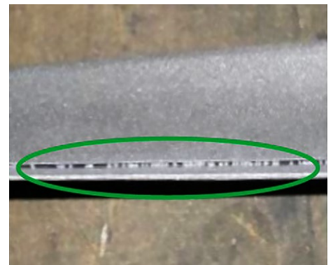
Figure 7: 20 mesh alumina grit trapped in a turbine blade trailing edge cooling slot
