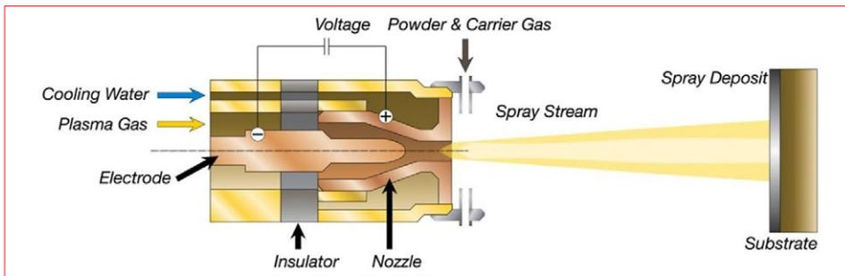
Figure 11: The (traditional) air plasma spray process
