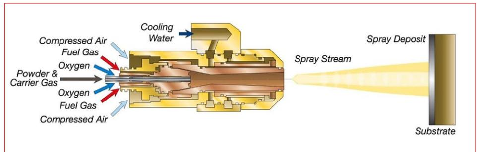
Figure 8: The HVOF gas fuel (HVOF-GF) process
