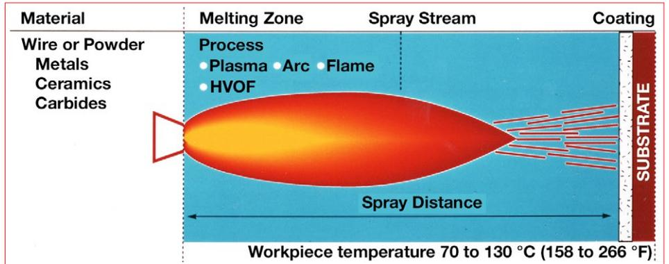
Figure 5: The basic principles of the thermal spray process
