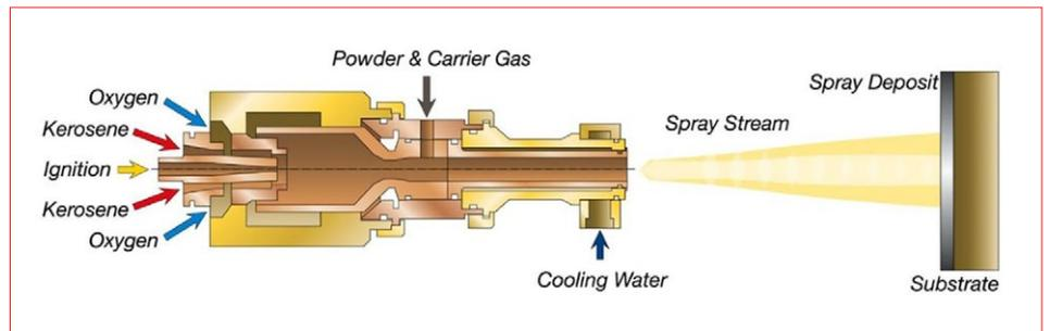
Figure 9: The HVOF liquid fuel (HVOF-LF) process
