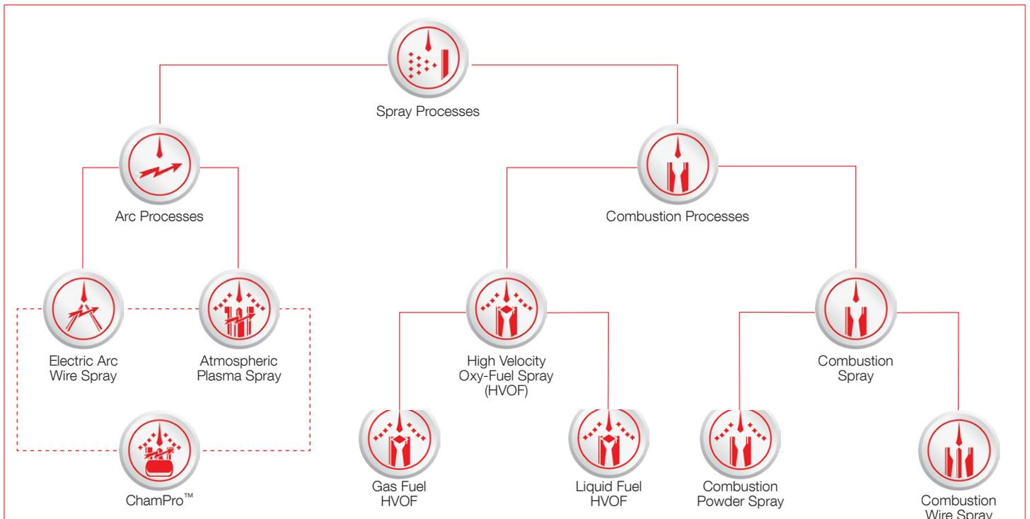
Figure 4: Overview of the main thermal spray processes.
