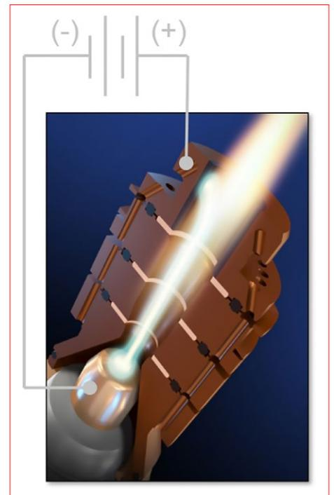
Figure 12: Cascaded arc plasma spray hardware cross-section
