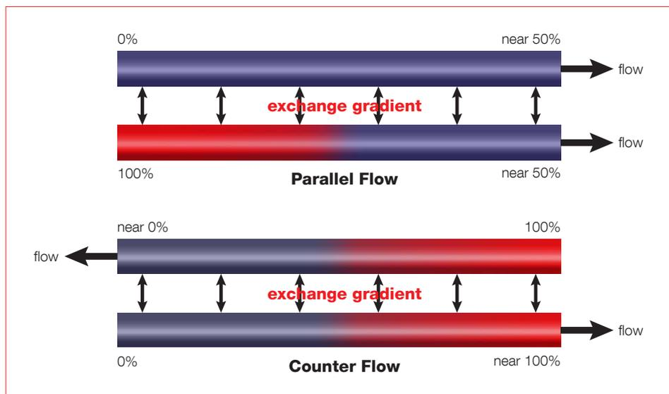
Figure 1. Comparison of parallel flow (top) and counter flow (bottom) heat transfer. Counter flow is much more efficient
