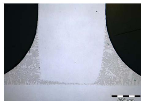
Figure 3. Brazed joint on a T-specimen (Amdry 105)
