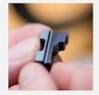
The chip formation was improved, although there was still a need for optimisation with respect to chip breaking.
