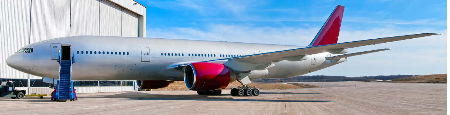
GE90-115B turbofan engines power the Boeing 777-200LR aircraft
