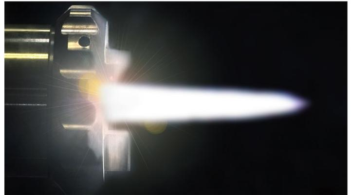
The Oerlikon Metco TriplexPro-210 plasma spray gun with high enthalpy flame.
