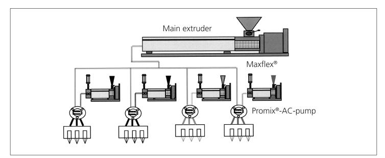
Figure 5: Additive supply by MAXFLEX® system extruder spinning
