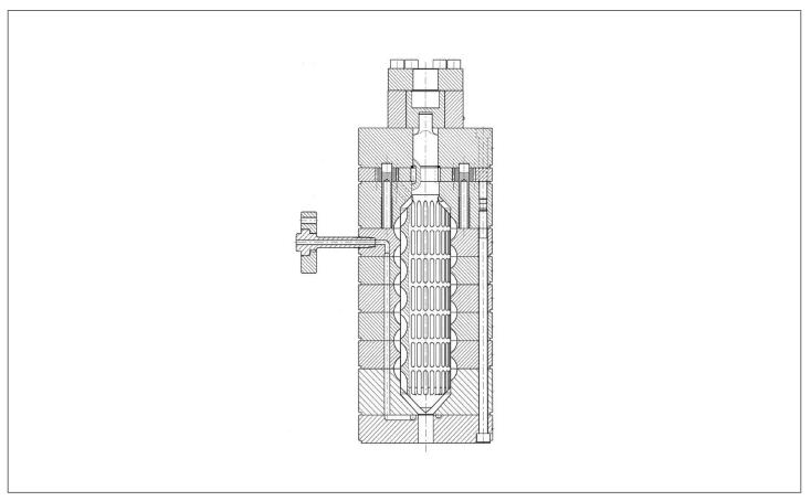
Figure 6: PROMIX® AC Melt spinning pump
