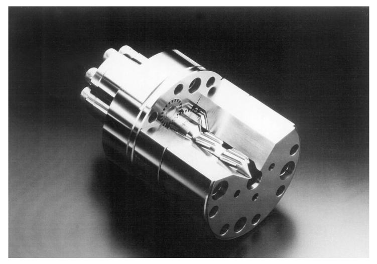
If a PROMIX<sup>®</sup> planetary-gear spin pump is used, the mixer of the pump shaft protrudin into the inlet ensures optimal melt quality in each individual stream. Differences in temperature and viscosity are minimized which, in turn, leads to greater uniformity in yarn properties as well as lower yarn break rates.
