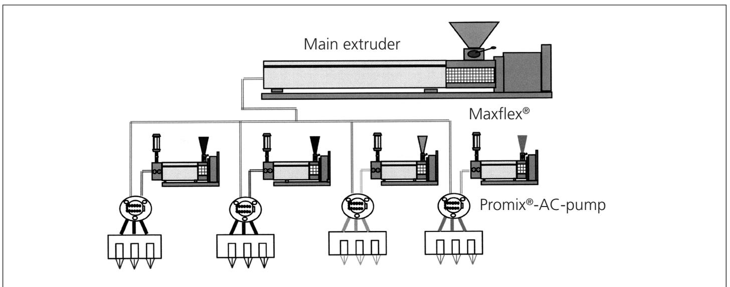
Figure 5: Additive supply by MAXFLEX® system extruder spinning
