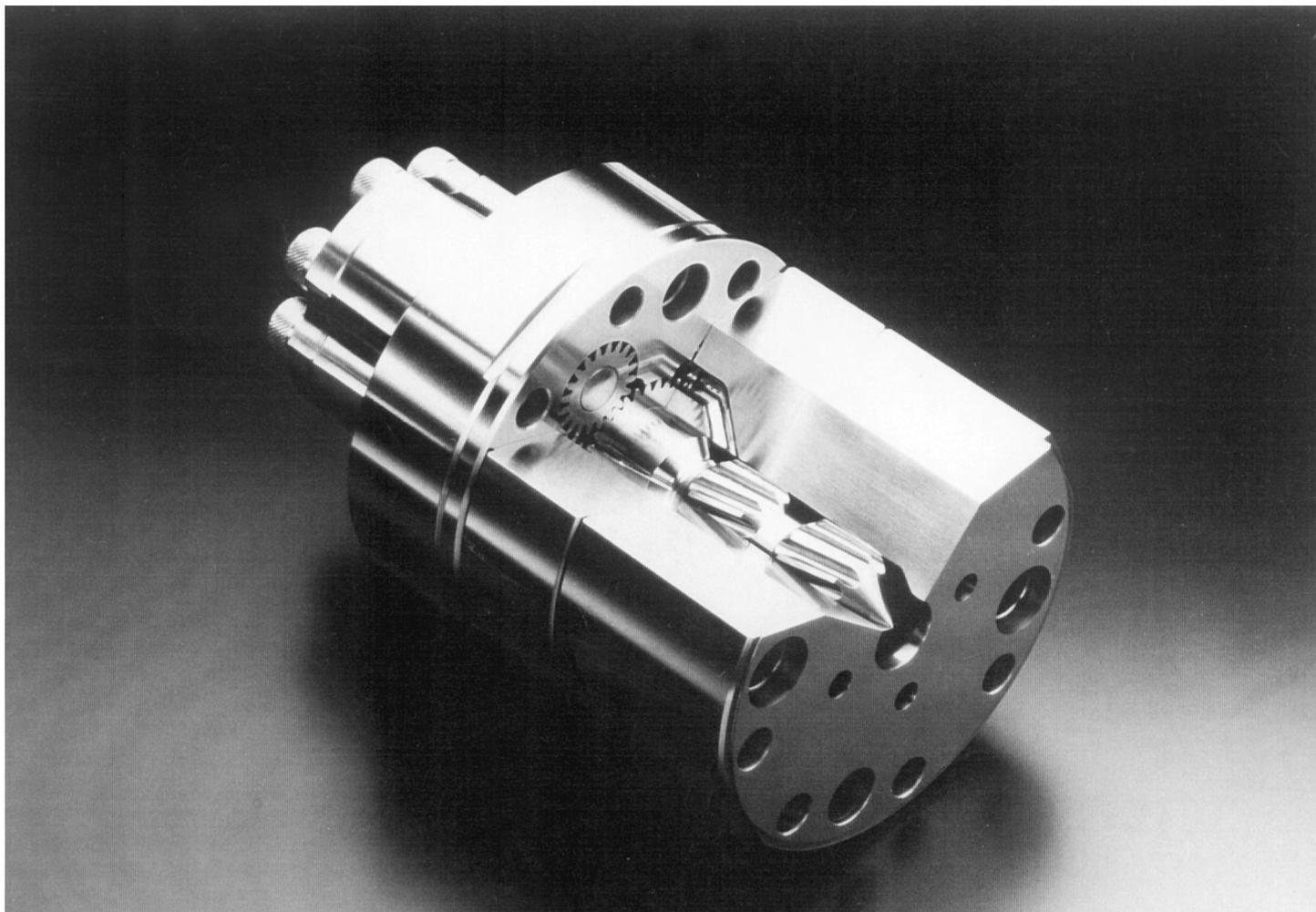
If a PROMIX® planetary-gear spin pump is used, the mixer of the pump shaft protrudes into the inlet ensuring optimal melt quality in each individual stream. Differences in temperature and viscosity are minimized which, in turn, leads to greater uniformity in yarn properties as well as lower yarn break rates.
