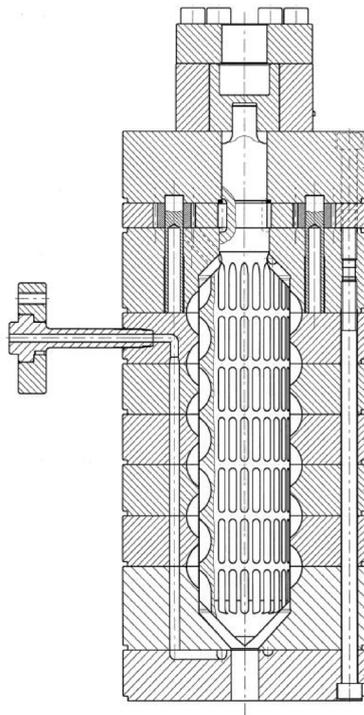
Figure 6: PROMIX® AC Melt spinning pump
