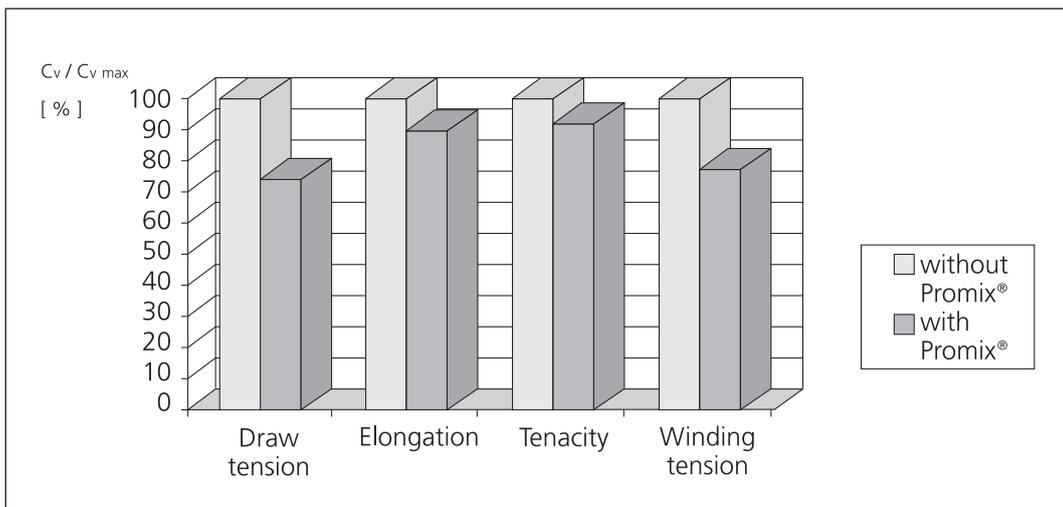
Figure 3: PROMIX® planetary gear pump - influence on yarn breaks
