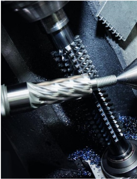
In hobbing, BALINIT ALTENZA allows even higher cutting speeds to be realized. / Figure: Oerlikon Balzers.
