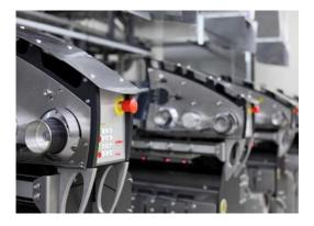
**Caption:** A new driver unit for WINGS POY further reduces the energy consumption in the winder section by 3%.
