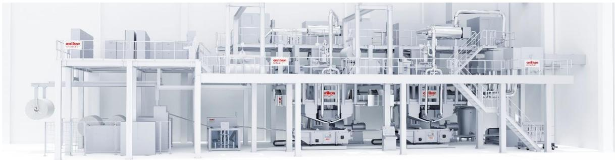
**Caption:** Oerlikon Nonwoven double-beam meltblown system – here with integrated ecuTEC+ for electrostatically-charging the filter media.
