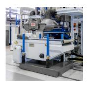
Oerlikon Neumag is premiering its new multifunctional forming table for its meltblown systems with a considerably reduced footprint and a shortened wire length that reduce maintenance costs.
