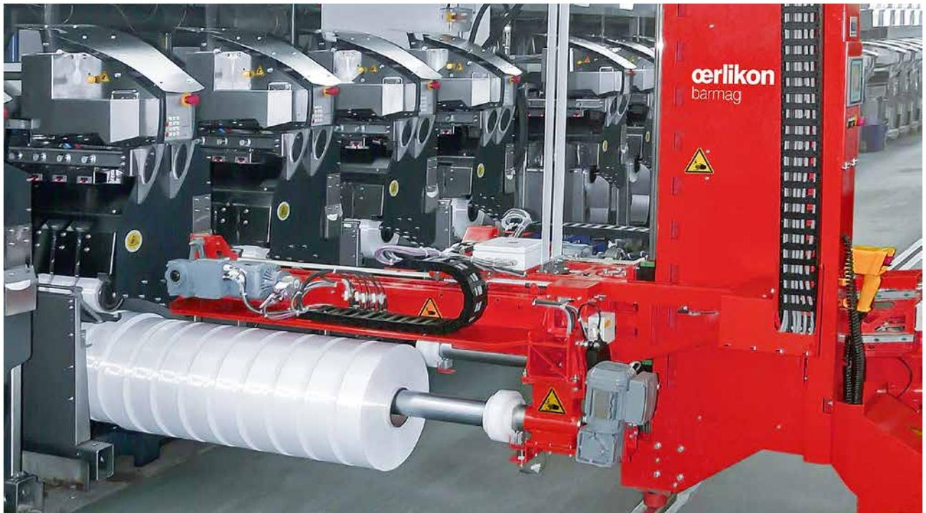
Oerlikon Barmag's Doffing system offers higher operating safety in sensitive working areas.
