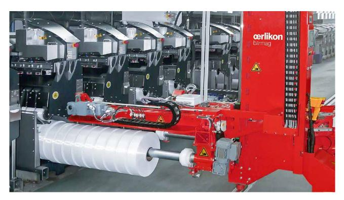
Oerlikon Barmag's Doffing system offers higher operating safety in sensitive working areas.
