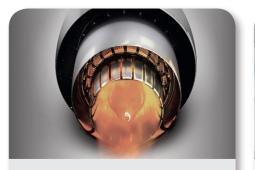
**Resist high temperatures** Thermal barrier coatings used in combustor and turbine sections of engines protect underlying materials from temperatures that these substrates could otherwise not tolerate.
