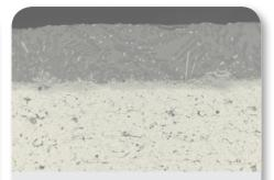
Innovative solutions to resist attack New materials continually being developed to arrest coating degradation caused by CMAS; allowing engines to operate longer in harsh environments.
