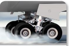
Ensure safe landings Landing gears coated with our highvelocity oxygen fuel thermal spray technology achieve superior performance and safety. These coatings replace the noxious hard chromium process.
